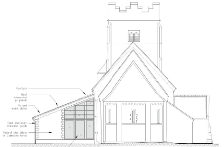
East Elevation Scale 1:100
