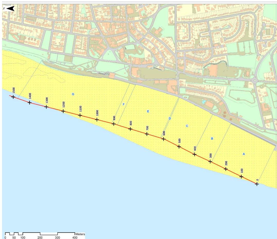
Figure 3-1 Hunstanton Frontage Chainage and Defence Sections
